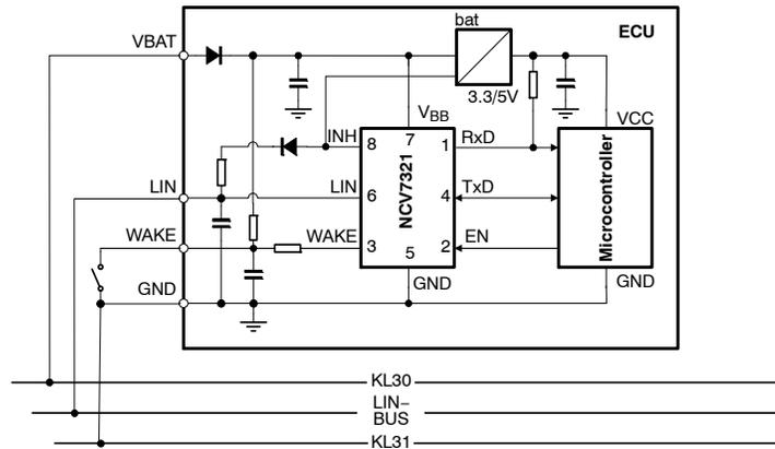
Figure 2. Typical Application Diagram for a Master Node
