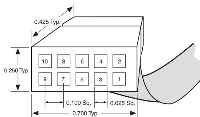
Dimensions are shown in inches. Spacing between pin centers is 0.1 inches.
