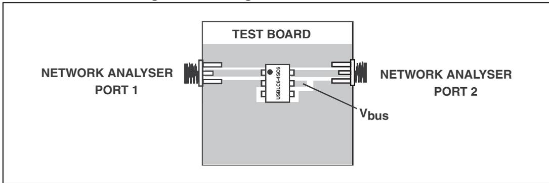
Figure 12. shows the measurement circuit for the analog application. In usual frequency range of analog signals (up to 240 MHz) the effect on disturbed line is less than -55 dB (see Figure 13.).
