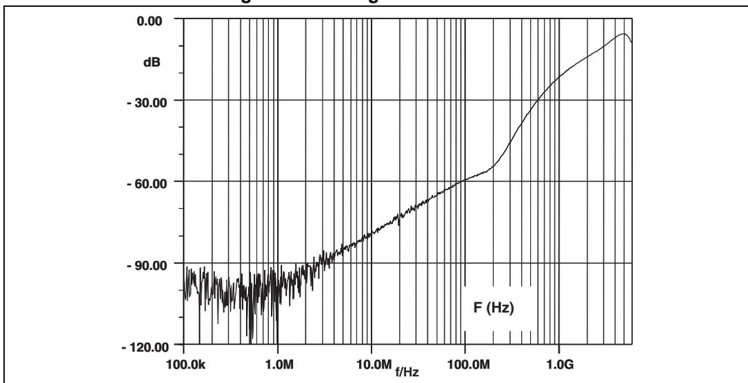
As the USBLC6-4SC6 is designed to protect high speed data lines, it must ensure a good transmission of operating signals. The frequency response (Figure 5.) gives attenuation information and shows that the USBLC6-4SC6 is well suitable for data line transmission up to 480 Mbit/s while it works as a filter for undesirable signals like GSM (900 MHz) frequencies, for instance.
