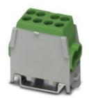
Trunk line branch terminal, Connection method: Screw connection, Screw connection, Number of connections: 4, Number of positions: 1, Cross section: 1.5 mm² - 25 mm², AWG: 8 - 2, Width: 23 mm, Color: green, Mounting type: NS 35/7,5, NS 35/15
