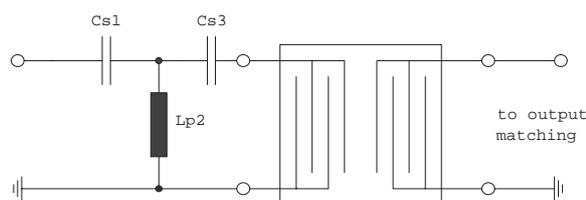
**Fig. 3 3<sup>rd</sup> order high-pass structure for basic ESD protection**
