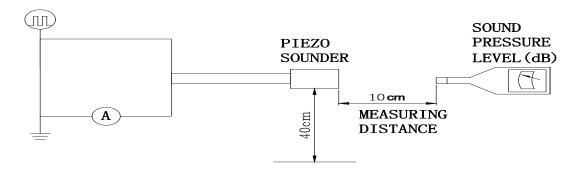
In the measuring test, buzzer is placed as follows:
