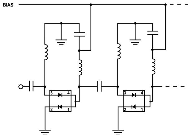
Figure 10. High Isolation SPST Switch (Repeat Cells as Required).
