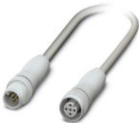
Sensor/Actuator cable, 5-position, PP-EPDM halogen-free, Gray RAL 7035, Plug straight M12, A-coded, on Socket straight M12, A-coded, Cable length: 0.6 m, Hygienic design, with plastic knurl
