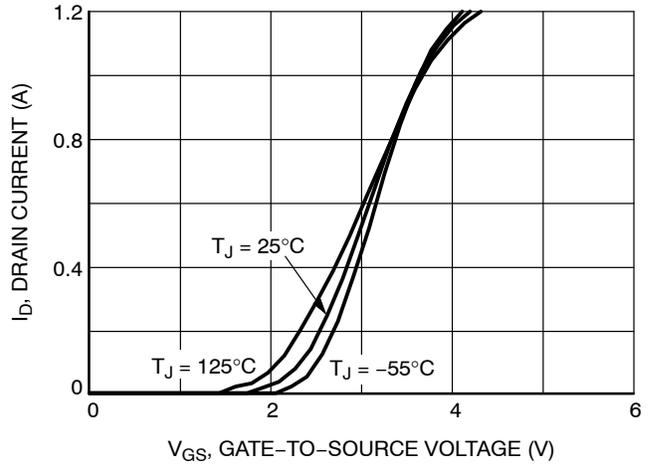
Figure 2. Transfer Characteristics
