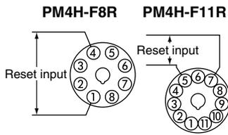
Use a contact with good contact reliability for the input. Contact bounce can lead to erroneous operation of the timer, so use a contact with short bounce time. Make the resistance between terminals for a short circuit less than 1k-ohms. Make the resistance between terminals for an open circuit greater than 100k-ohms.
