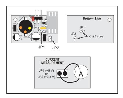
Figure B-5. Prototyping Board Current-Measurement Option
