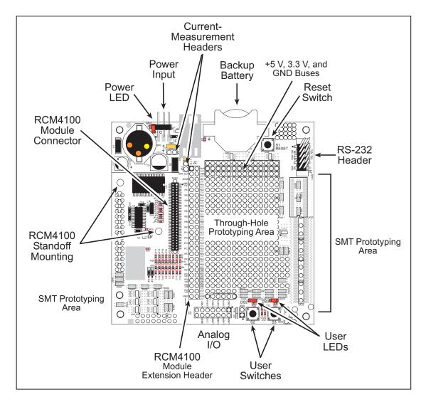
Figure B-1. Prototyping Board
