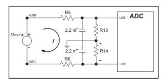
Figure 10. Current Flow from Ungrounded or Floating Source
