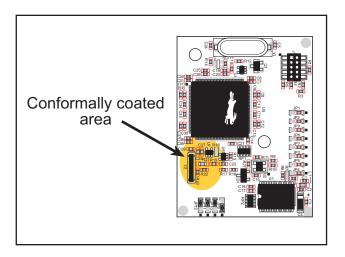
Figure A-6. RCM4100 Areas Receiving Conformal Coating
