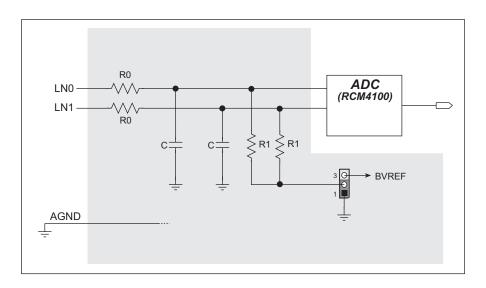
Figure 9. Resistor Divider Network for Analog Inputs
