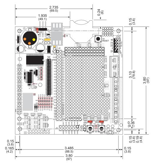
Figure B-2. Prototyping Board Dimensions
