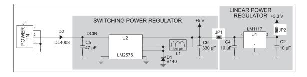
Figure B-3. Prototyping Board Power Supply
