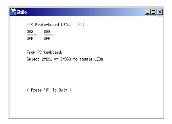
Press "2" or "3" on your keyboard to select LED DS2 or DS3 on the Prototyping Board. Then follow the prompt in the Dynamic C **STDIO** window to turn the LED ON or OFF. A logic low will light up the LED you selected.
