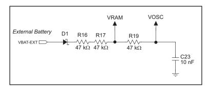
Figure C-2. RCM4100 Backup Battery Circuit
