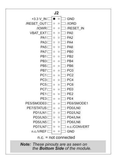
Figure 6. RCM4100 Series Pinout
