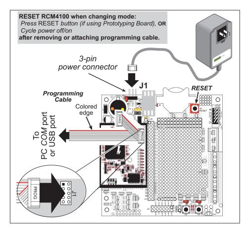
Figure 8. Switching Between Program Mode and Run Mode
