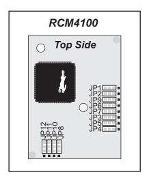
Figure A-5. Location of RCM4100 Configurable Positions
