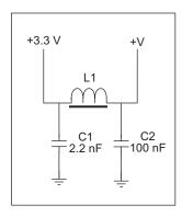
Figure 12. Analog Supply Circuit
