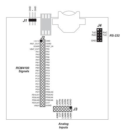
Figure B-4. Prototyping Board Pinout
