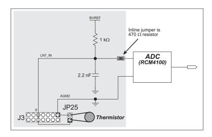
Figure B-7. Prototyping Board Thermistor Input
