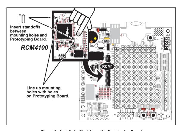
Figure 3. Install the Module on the Prototyping Board
