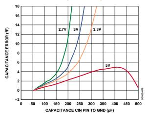
Figure 10. Capacitance Input Error vs. Capacitance between CIN and GND, CIN(+) to EXC = 21 pF, CIN(-) to EXC = 23 pF,  $V_{DD} = 2.7 \text{ V}$ , 3 V, 3.3 V, and 5 V, the Same Configuration as in Figure 34
