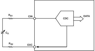
Figure 39. Parasitic Serial Resistance
