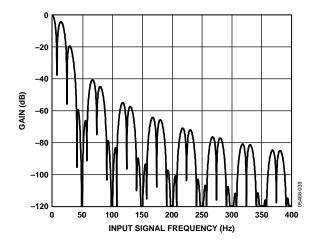
Figure 23. Voltage Channel Frequency Response, Conversion Time = 122.1 ms
