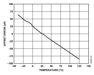
Figure 8. Capacitance Input Gain Drift vs. Temperature,  $V_{DD} = 5 V$ , CIN(+) to EXC = 4 pF, the Same Configuration as in Figure 30
