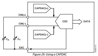
The CAPDAC can be understood as a negative capacitance connected internally to the CIN pin. There are two independent CAPDACs, one connected to the CIN(+) and the second connected to the CIN(-). The relation between the capacitance input and output data can be expressed as
