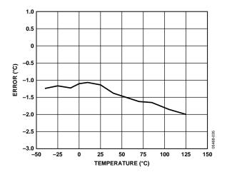
Figure 19. External Temperature Sensor Error vs. Temperature
