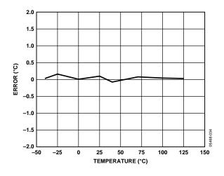
Figure 18. Internal Temperature Sensor Error vs. Temperature
