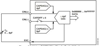
Figure 31. Using CAPDAC in Single-Ended Mode
