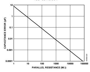
Figure 14. Capacitance Input Error vs. Resistance in Parallel with Measured Capacitance
