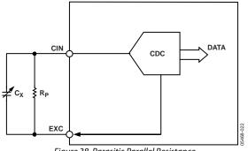
Figure 38. Parasitic Parallel Resistance
