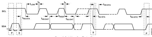
Figure 3. Serial Interface Timing Diagram
