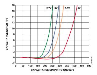
Figure 9. Capacitance Input Error vs. Capacitance between CIN and GND. CIN(+) to EXC = 4 pF, CIN(-) to EXC = 0 pF, V<sub>DD</sub> = 2.7 V, 3 V, 3.3 V, and 5 V, the Same Configuration as in Figure 33
