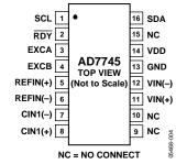
Figure 4. AD7745 Pin Configuration (16-Lead TSSOP)
