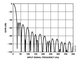
Figure 22. Capacitance Channel Frequency Response, Conversion Time = 109.6 ms
