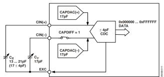
Figure 35. Using CAPDAC in Differential Mode
