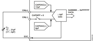
Figure 32. Using CAPDAC in Single-Ended Mode
