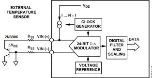
Figure 41. Transistor as an External Temperature Sensor
