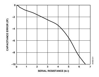
Figure 15. Capacitance Input Error vs. Serial Resistance, CIN(+) to EXC = 21 pF, CIN(-) to EXC = 23 pF,  $V_{DD} = 5 \text{ V}$ , the Same Configuration as in Figure 34.
