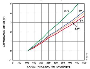
Figure 11. Capacitance Input Error vs. Capacitance between EXC and GND, CIN(+) to EXC = 21 pF, CIN(-) to EXC = 23 pF,  $V_{DD} = 2.7 \text{ V}$ , 3 V, 3.3 V, and 5 V, the Same Configuration as in Figure 34
