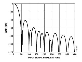
Figure 21. Capacitance Channel Frequency Response, Conversion Time = 62 ms
