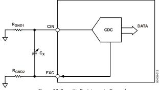
Figure 37. Parasitic Resistance to Ground
