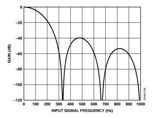
Figure 20. Capacitance Channel Frequency Response, Conversion Time = 11 ms
