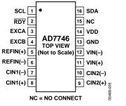
Figure 5. AD7746 Pin Configuration (16-Lead TSSOP)
