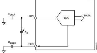
Figure 36. Parasitic Capacitance to Ground
