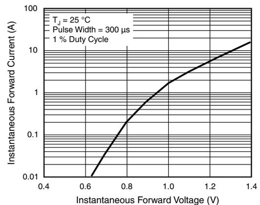
Fig. 4 - Typical Forward Characteristics Per Diode
