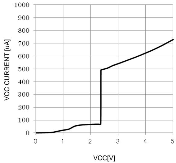
Figure 15. VCC input current vs VCC (STB ON)
