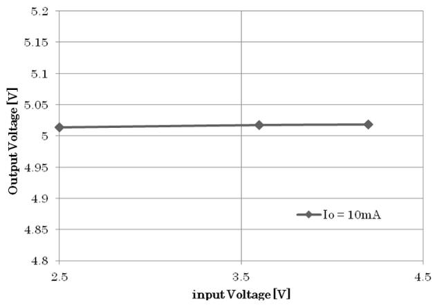
Figure 25. CH2 Output voltage vs Input voltage
