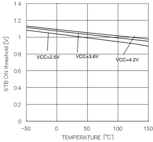
Figure 8. STB ON threshold voltage vs temp
