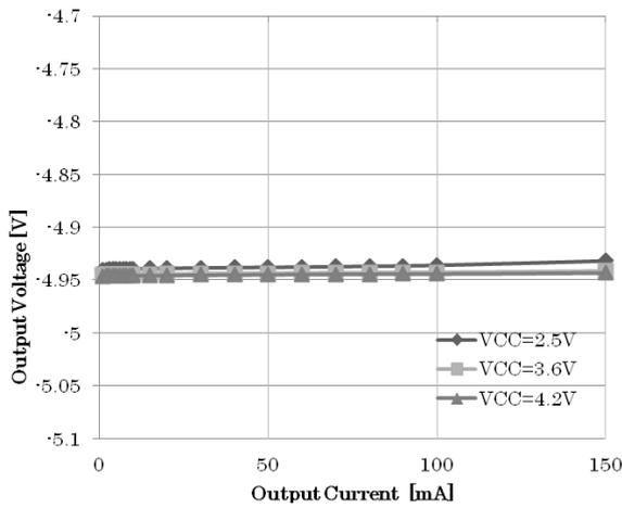
Figure 22. CH1 Output voltage vs Output Current
