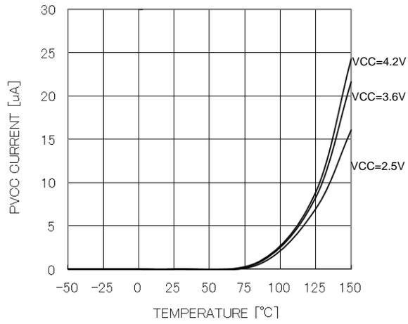
Figure 16. VCC input current vs Temp (STB OFF)
