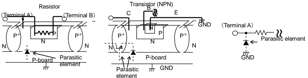
Figure 35. Simplified structure of a Bipolar IC
