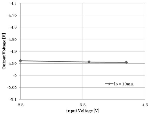
Figure 24. CH1 Output voltage vs Input voltage
