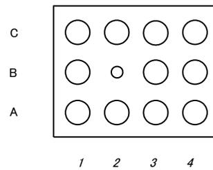
Figure 2. Pin assignment (Bottom view)
