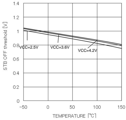
Figure 9. STB OFF threshold voltage vs temp
