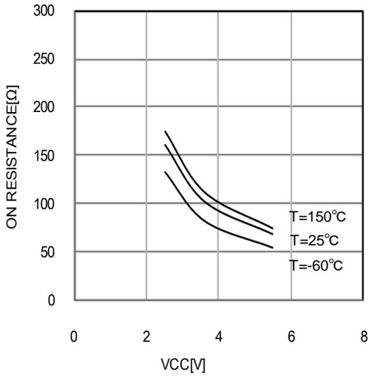
Figure 14. NON1 discharge SW ON resistance vs VCC
