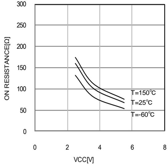
Figure 13. DIS1 discharge SW ON resistance vs VCC
