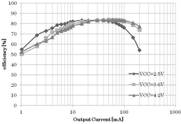
Figure 20. CH1 Power conversion efficiency vs output current
