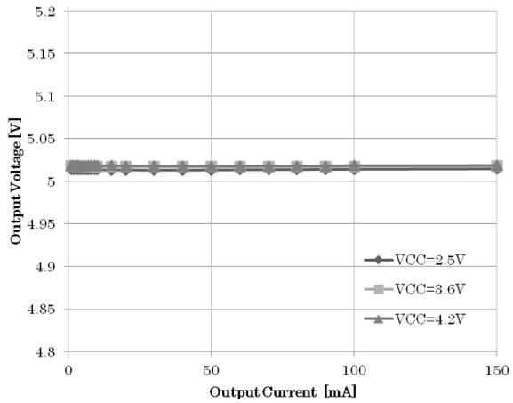
Figure 23. CH2 Output voltage vs Output Current
