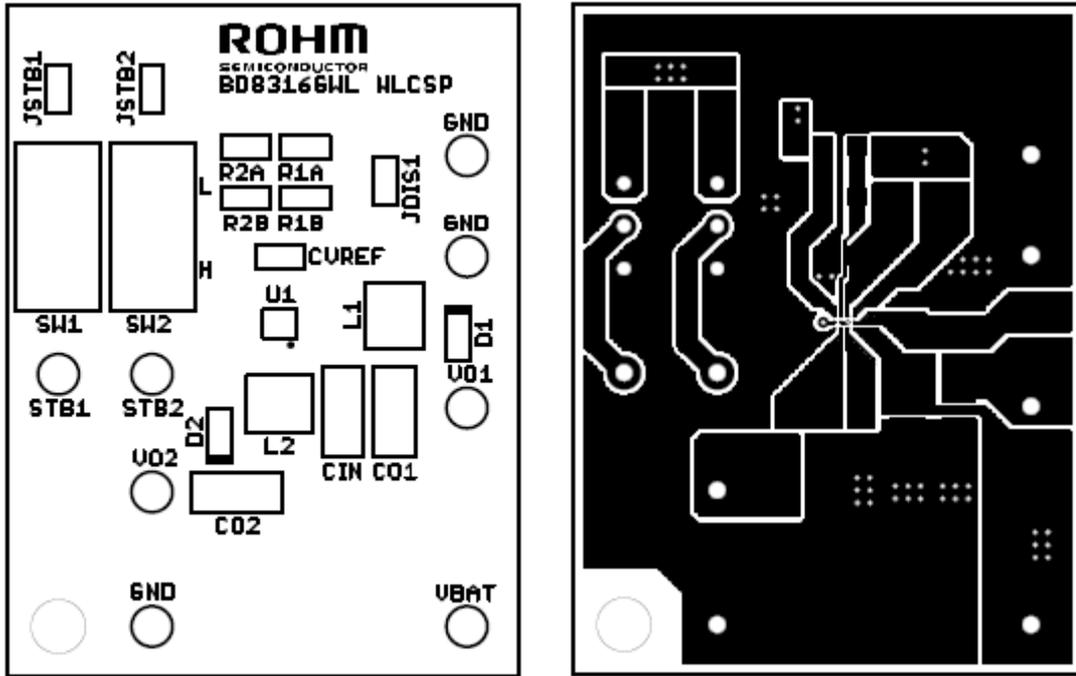
Figure 18. Assembly Layer
