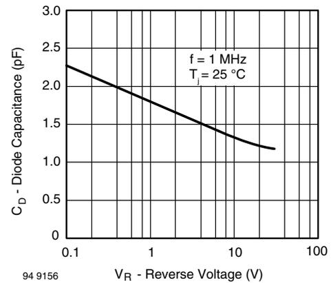
Fig. 3 - Diode Capacitance vs. Reverse Voltage
