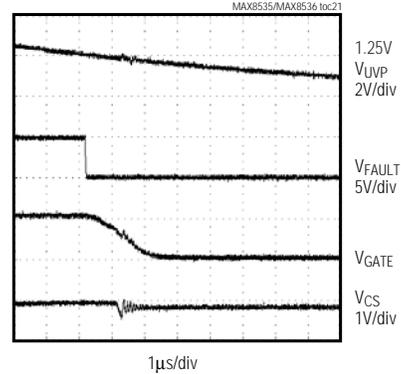
**SELECTIVE OVP SHUTDOWN WAVEFORM ( $R_1 = 10\Omega$ )**
