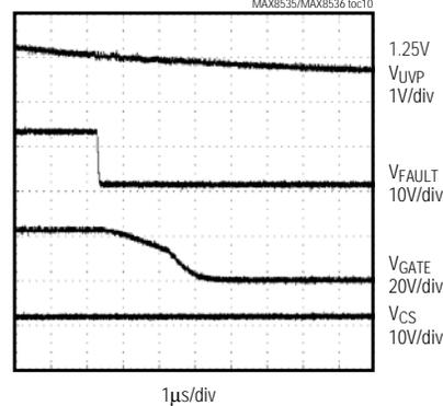
**SELECTIVE OVP SHUTDOWN WAVEFORM ( $R_1 = 10\Omega$ )**
