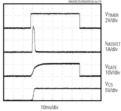
**REVERSE-CURRENT FAULT WAVEFORM ( $R_1 = 10\Omega$ )**
