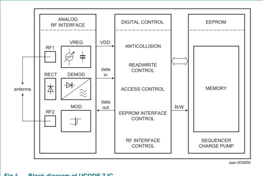
Fig 1. Block diagram of UCODE 7 IC
