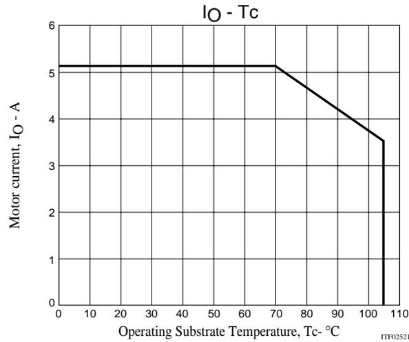
The motor current,  $I_O$ , shown above represents the range of DC operation and chopping operation.
