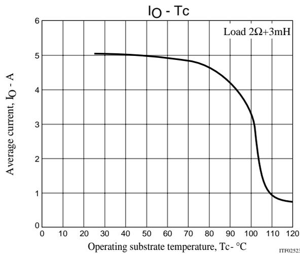
Overheating current control functions to prevent driver failure if a motor lock malfunction occurs.
