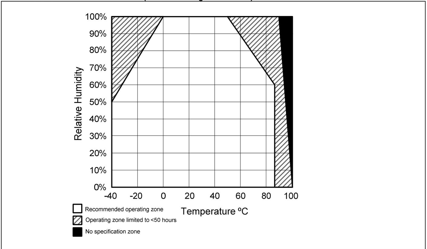
**FIGURE 2. STORAGE ENVIRONMENT (Non-condensing environment.)**
