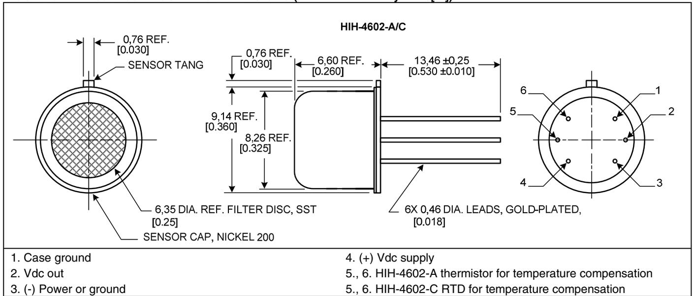
**FIGURE 6. RH SENSOR CONSTRUCTION**
