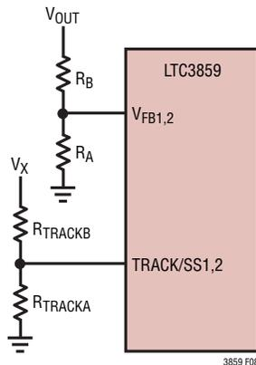
Figure 8. Using the TRACK/SS Pin for Tracking
