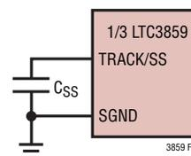
Figure 6. Using the TRACK/SS Pin to Program Soft-Start
