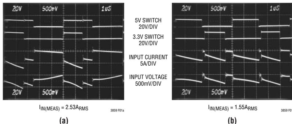
**Figure 1. Input Waveforms Comparing Single-Phase (a) and 2-Phase (b) Operation for Dual Switching Regulators Converting 12V to 5V and 3.3V at 3A Each. The Reduced Input Ripple with the 2-Phase Regulator Allows Less Expensive Input Capacitors, Reduces Shielding Requirements for EMI and Improves Efficiency**
