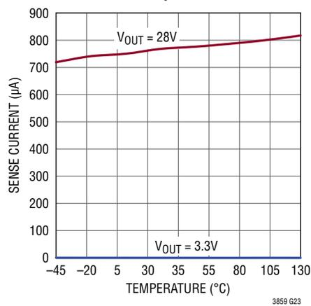
**Boost SENSE Pin Total Input Current vs Temperature**
