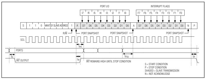
Figure 7. Reading the MAX7321 (2 Data Bytes)
