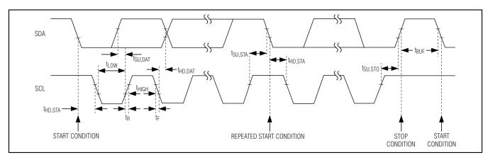
Figure 1. 2-Wire Serial Interface Timing Details
