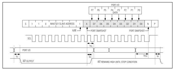
Figure 6. Reading the MAX7321 (1 Data Byte)
