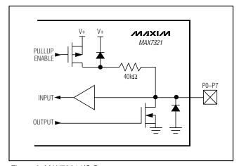
Figure 9. MAX7321 I/O Structure
