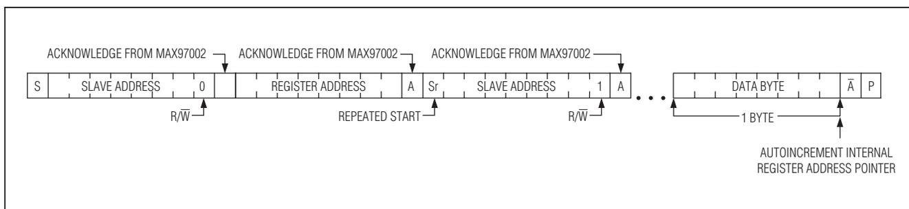
Figure 13. Reading n-Bytes of Data from the MAX97002
