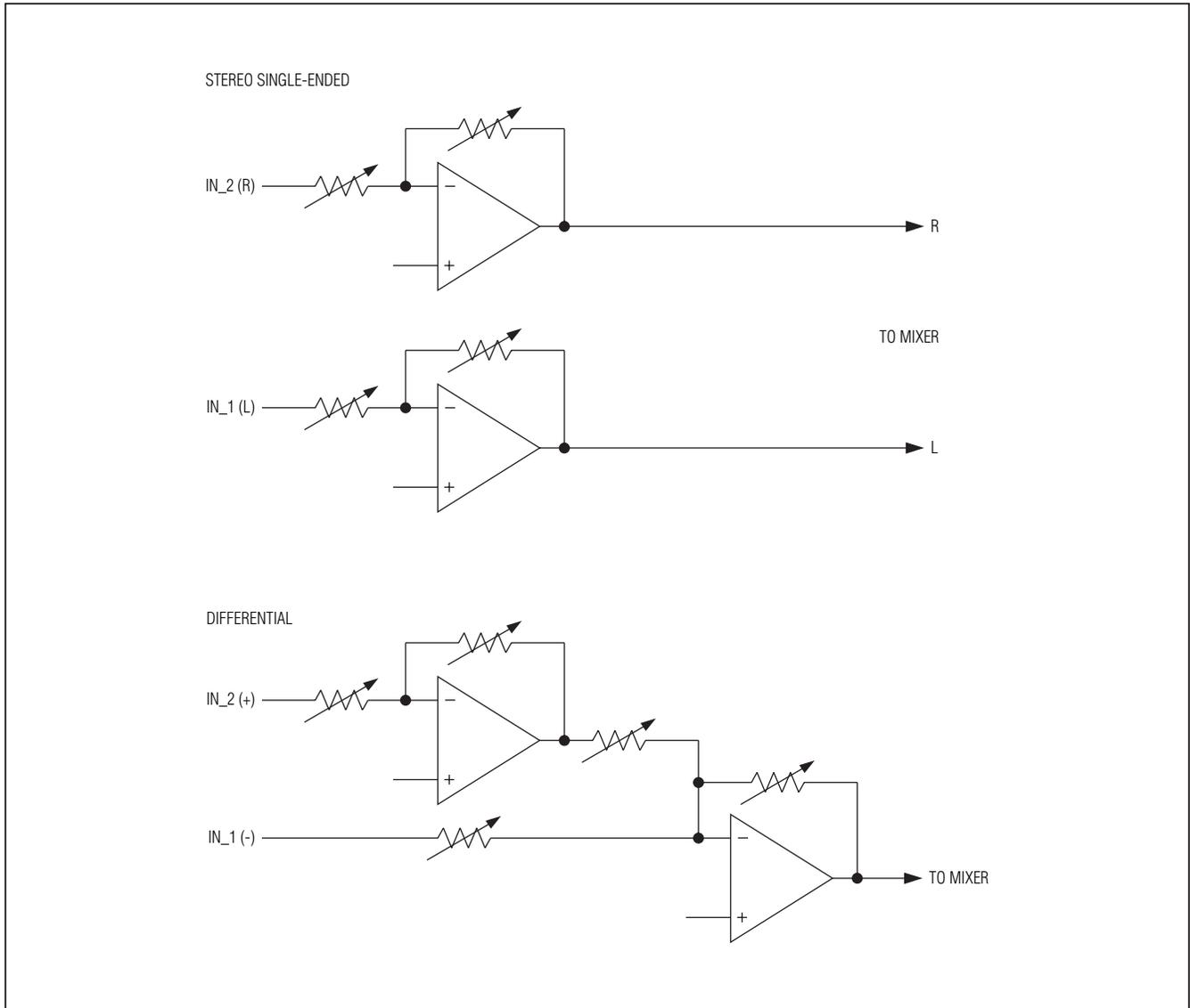
Figure 3. Differential and Stereo Single-Ended Input Configurations
