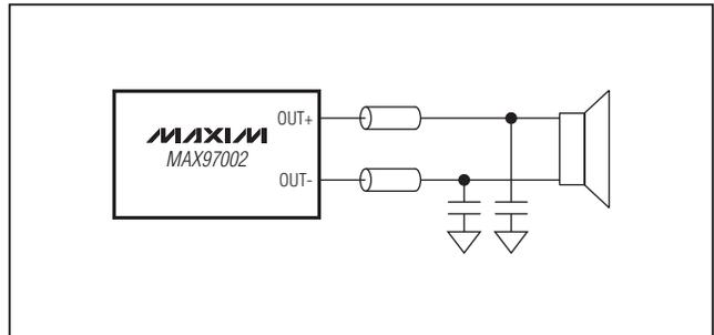
Figure 14. Optional Class D Ferrite Bead Filter
