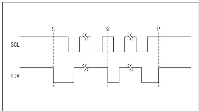
Figure 8. START, STOP, and REPEATED START Conditions
