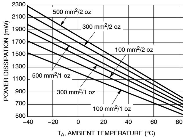
**Figure 7. Power Dissipation vs. Ambient Temperature @  $T_J = 150^\circ\text{C}$**
