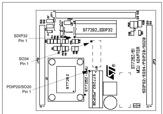
Figure 14: SO34/SDIP32/PDIP20/SO20 pin 1 location
