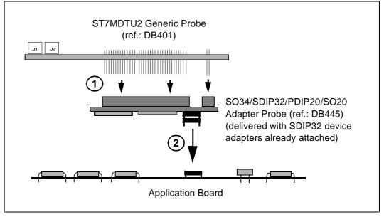
Figure 15: SDIP32 MCU package connections
