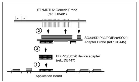
Figure 16: PDIP20 MCU package connections
