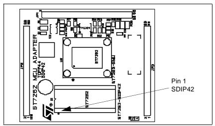
Figure 11: SDIP42 Pin 1 Location on TQFP44/SDIP42 adapter probe
