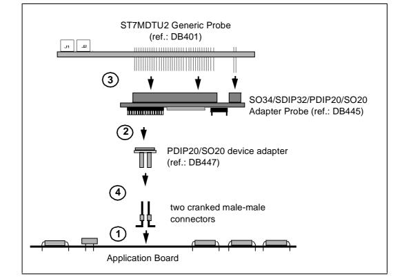
Figure 17: SO20 MCU package connections
