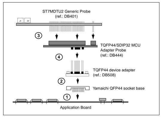
Figure 7: TQFP44 MCU package connections
