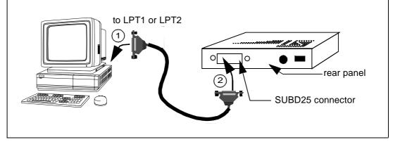
Figure 4: Connecting the emulator to the PC
