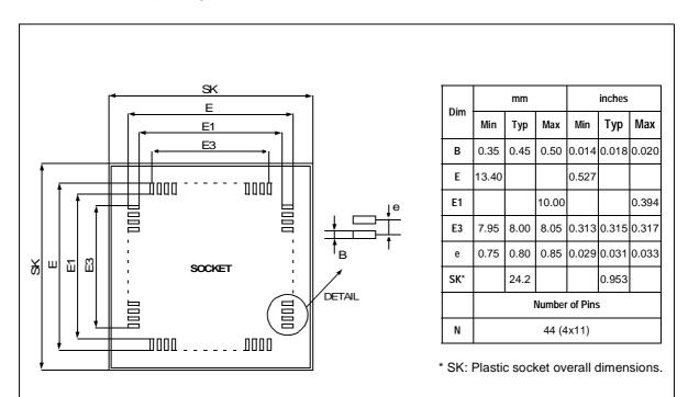
Figure 20: TQFP44 Device and emulation probe compatible footprint
