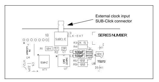
The SUB-click **external clock** connector on the probe can be used with the two SMB to BNC connectors provided in the emulator package. Voltage at these connectors must range between 0 V and 5 V. The levels are TTL.
