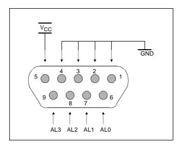
You can view these probe inputs using STVD7. From the main menu, select *View>Trace*. The input signal values are listed under the Sig column (AL3..0).
