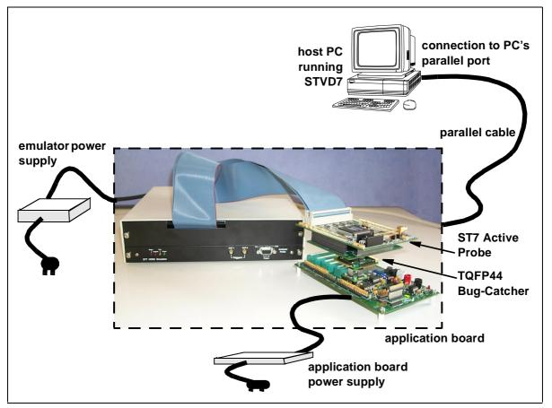
Figure 1: ST7MDTU2-EMU2B general configuration
