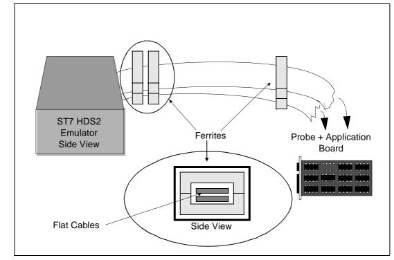
Figure 6: Making your probes EMC-compliant
