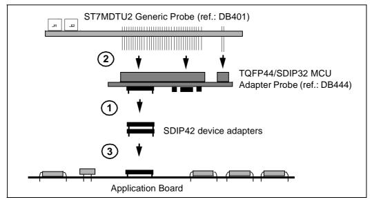
Figure 10: SDIP42 MCU package connections
