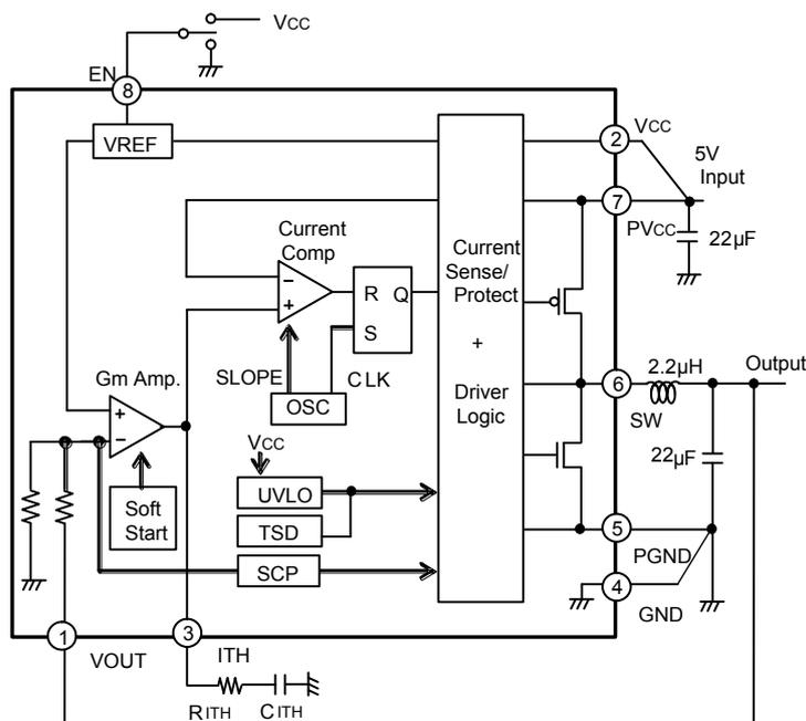
Fig.3 Block Diagram
