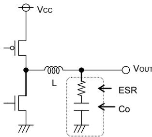
Fig.29 Output capacitor
