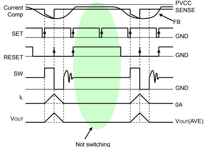
Fig.21 SLLM™ switching timing chart
