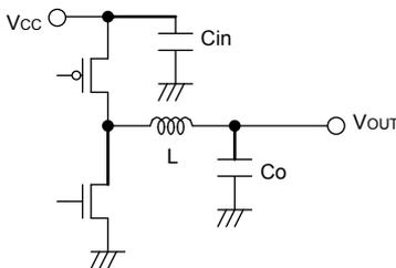
Fig.30 Input capacitor
