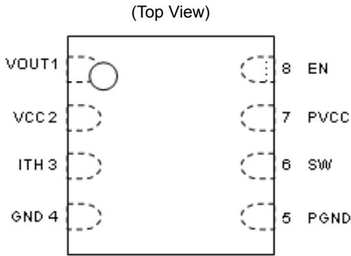
Fig.2 Pin Configuration
