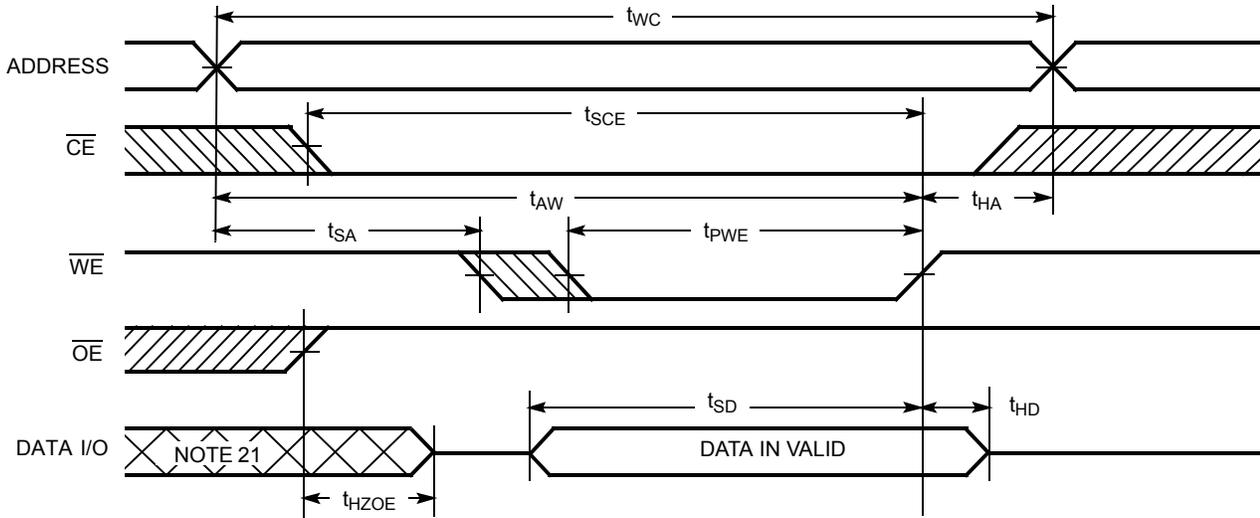
Figure 8. Write Cycle No. 3 ( $\overline{WE}$  Controlled,  $\overline{OE}$  LOW) [20]
