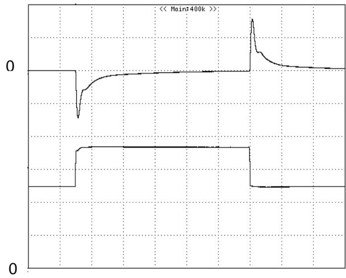
**Figure 9:** Output voltage response to step-change in load current (75%-50%-75% of  $I_o$ , max;  $di/dt = 2.5A/\mu s$ ). Load cap:  $470\mu F$ ,  $35m\Omega$  ESR solid electrolytic capacitor and  $1\mu F$  ceramic capacitor. Top Trace:  $V_{out}$  (50mV/div, 200us/div), Bottom Trace:  $I_{out}$  (5A/div). Scope measurement should be made using a BNC cable (length shorter than 20 inches). Position the load between 51 mm to 76 mm (2 inches to 3 inches) from the module
