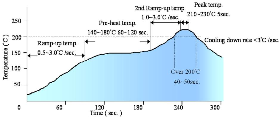
Note: The temperature refers to the pin of E48SR, measured on the pin +Vout joint.
