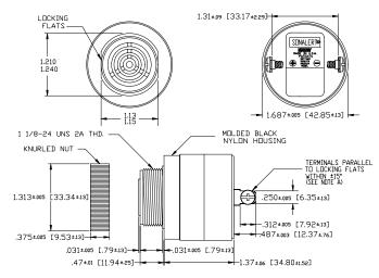
NOTE A: TERMINALS-032 BRASS TIN PLATED, TAPPED FOR #6-32 SCREW. TWO #6-32 NICKLE PLATED BRASS SCREWS INCLUDED. WILL ACCEPT 1/4\* QUICK CONNECT.
