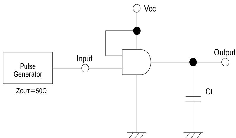
Note: Open output when measuring supply current
