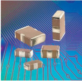
X2Y<sup>®</sup> filter capacitors employ a unique, patented low inductance design featuring two balanced capacitors that are immune to temperature, voltage and aging performance differences. These components offer superior decoupling and EMI filtering performance, virtually eliminate parasitics, and can replace multiple capacitors and inductors saving board space and reducing assembly costs.
