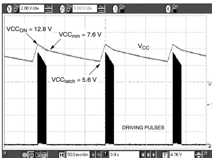
Figure 18. Typical Waveforms in Short Circuit Conditions
