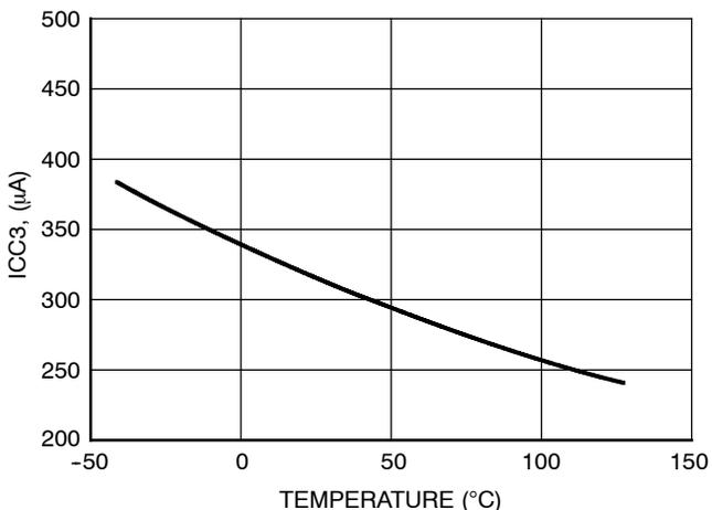
Figure 9. ICC<sub>3</sub> vs. Temperature
