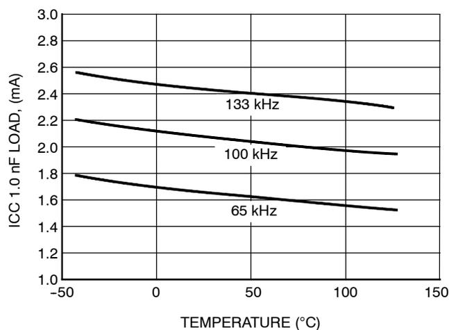
Figure 6. ICC 1.0 nF Load vs. Temperature
