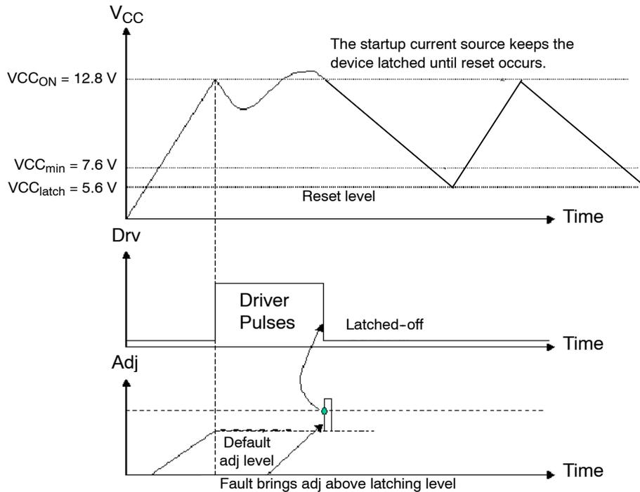
**Figure 24. When V<sub>adj</sub> is Pulled Above 3.1 V, NCP1217 Permanently Latches-Off the Output Pulses**
