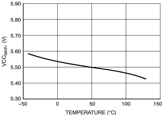
Figure 8. V<sub>CC\_latch</sub> vs. Temperature
