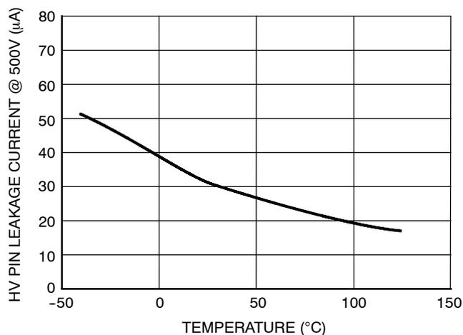
Figure 3. High Voltage Pin Leakage Current vs. Temperature
