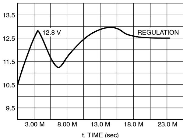
Figure 17. A Typical Startup Sequence for the NCP1217
