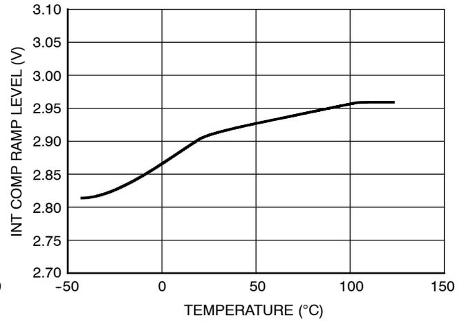
Figure 14. Int Comp Ramp Max Level vs. Temperature
