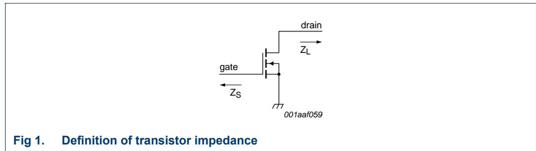
Fig 1. Definition of transistor impedance
