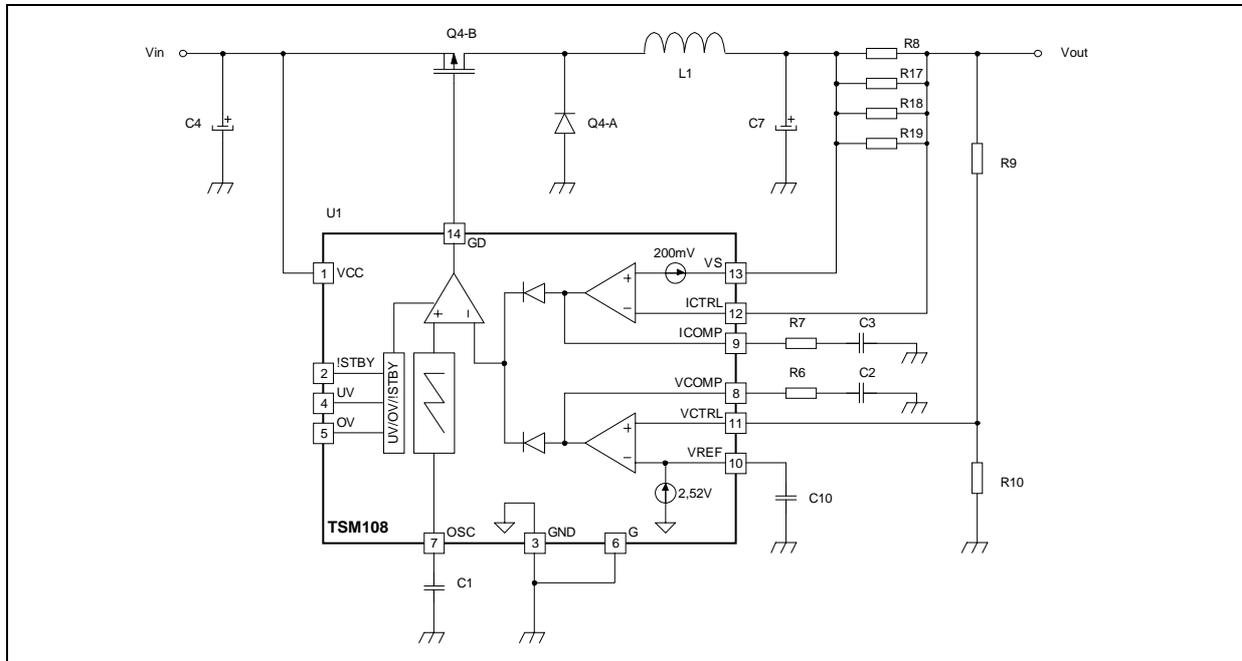
The list of components used in the typical application board is shown in the bill of material here below. All other components are not mounted. Passive components like capacitors and resistors used in this Evaluation Board are through-hole components to be more easily changed by the user. Of course, in real-life application, surface-mounted devices will be used and the whole application can fit into a very small PCB area.
