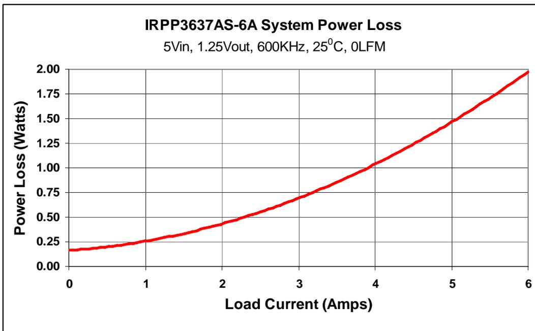
Figure 4b: IRPP3637-06A Reference Design Power Loss Curve
