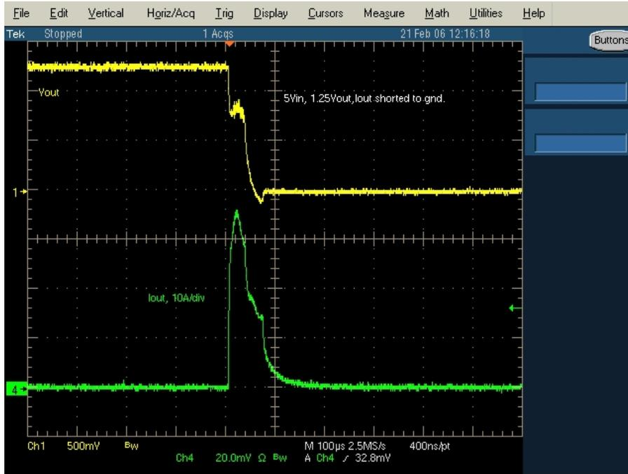
Figure 13: Output short circuit protection. Ch1=V<sub>OUT</sub>, Ch4=I<sub>OUT</sub>10A/div
