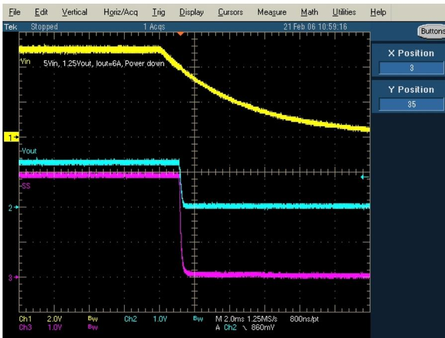
Figure 12: Power down. Ch1=V<sub>IN</sub>, Ch2=V<sub>OUT</sub>, Ch3=Soft Start
