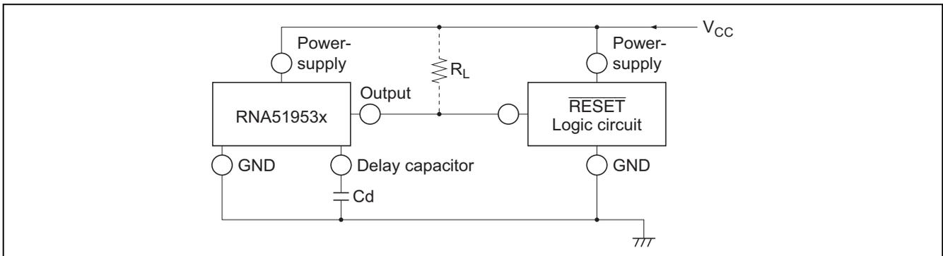
**Figure 1 Reset Circuit of RNA51953**
