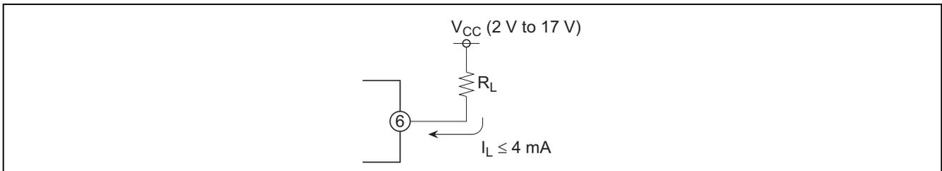
Figure 6 Output Load Resistance R<sub>L</sub>
