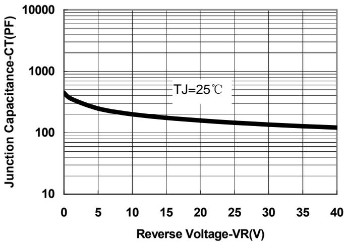
Fig.1-Typical Junction Capacitance
