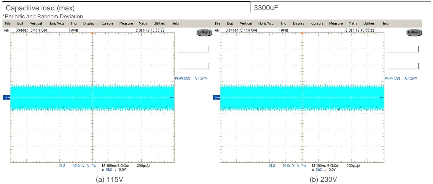
Fig. 2 Ripple & Noise example, 20MHz BW
