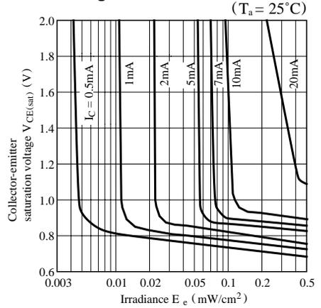
**Fig.9-b Collector-emitter Saturation Voltage vs. Irradiance (PT481F/PT483F1)**
