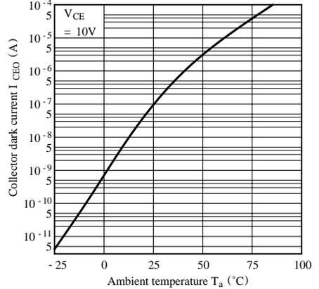
**Fig. 3 Relative Collector Current vs. Ambient Temperature**
