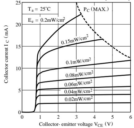
**Fig.5-b Collector Current vs. Collector-emitter Voltage**
