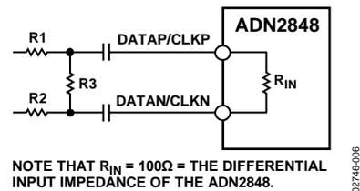
Figure 6. Attenuation Circuit
