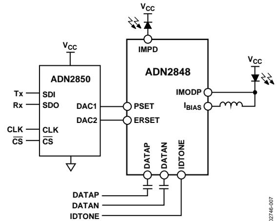
Figure 7. Application Using the ADN2850 Dual 10-Bit Digital Potentiometer with Extremely Low Temperature Coefficient as an Optical Supervisor
