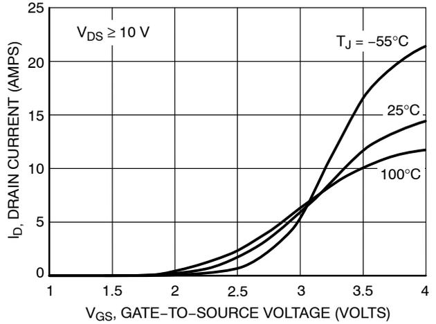
Figure 2. Transfer Characteristics
