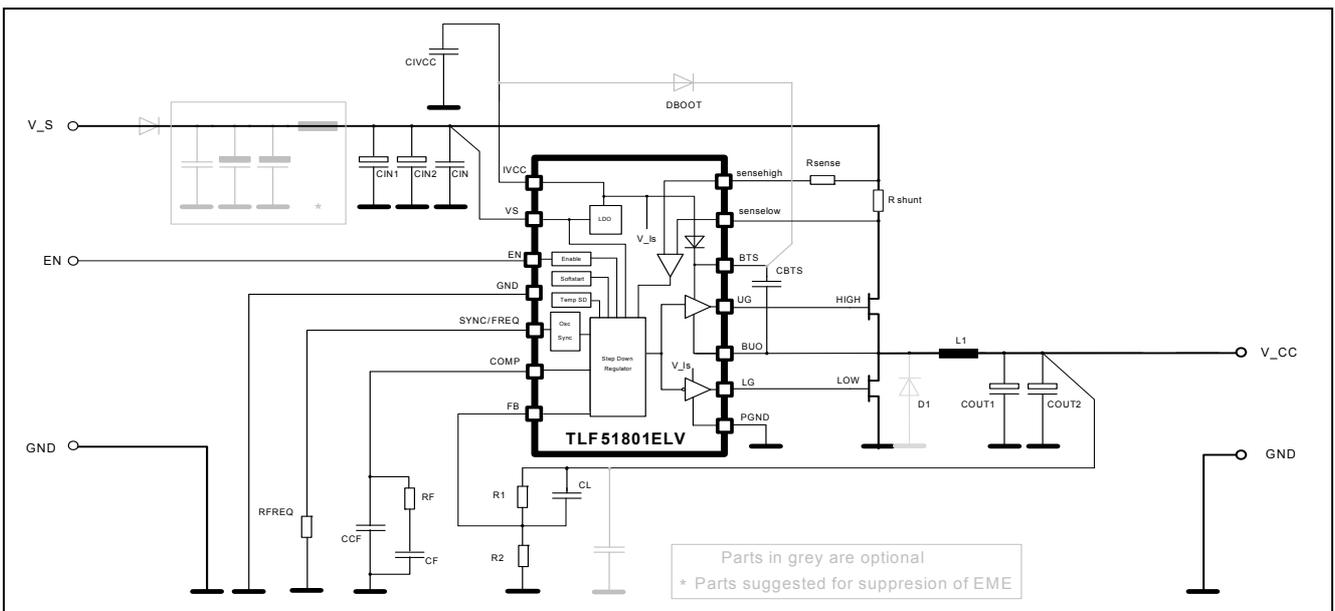
Figure 13 Application Diagram (Current limitation with Shunt-configuration)
