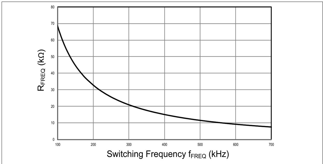
**Figure 10 Resistor R<sub>FREQ</sub> versus Switching Frequency f<sub>FREQ</sub>**
