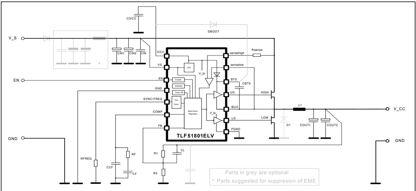
Figure 12 Application Diagram (Current limitation with Rdson-configuration)
