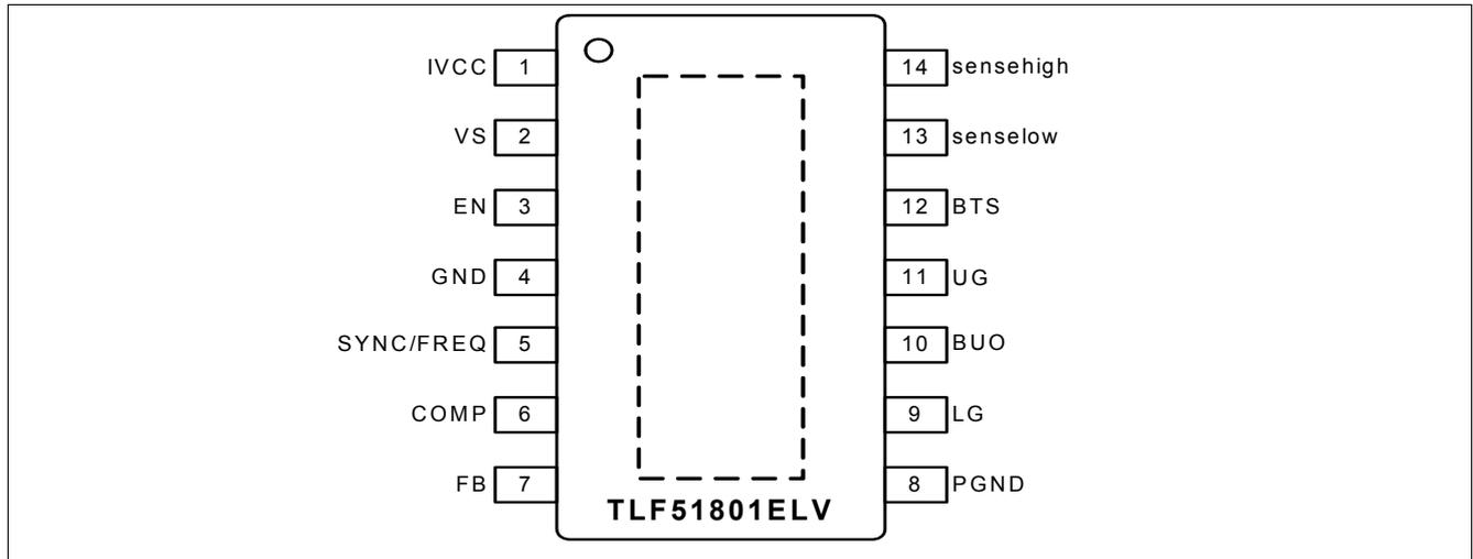
Figure 2 Pin Configuration
