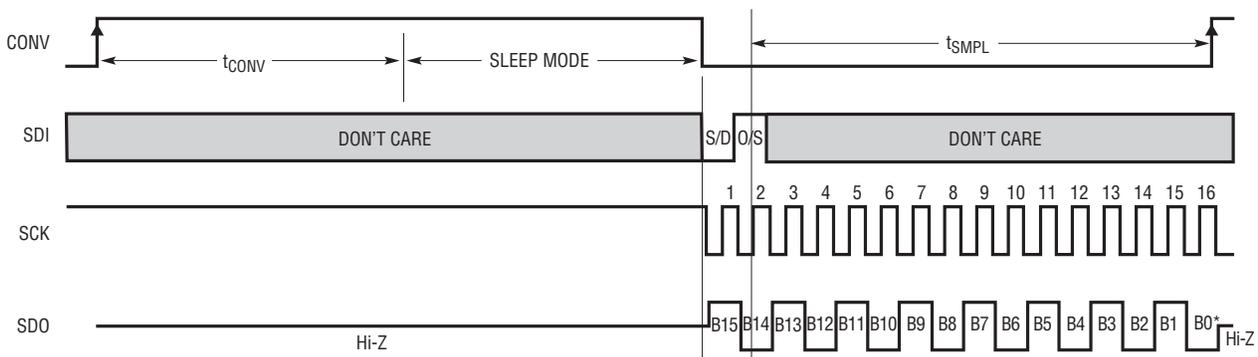
\*AFTER COMPLETING THE DATA TRANSFER, IF FURTHER SCK CLOCKS ARE APPLIED WITH CONV LOW, THE ADC WILL OUTPUT ZEROS INDEFINITELY
