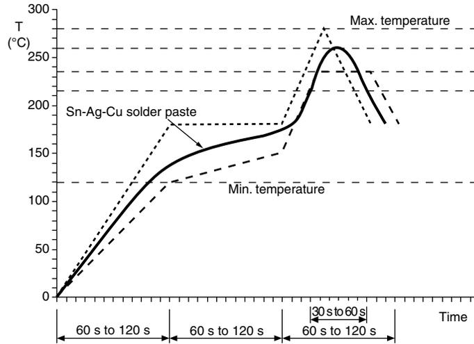
Fig. 8 - Soldering IR Reflow with SnAgCu Solder
