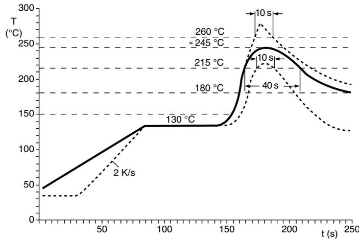
Fig. 7 - Soldering Reflow with Sn Solder
