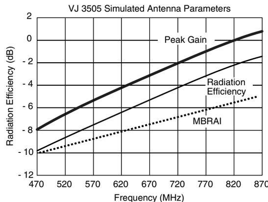
Fig. 1 - Peak Gain and Efficiency vs. Frequency
