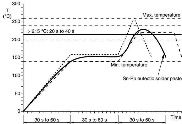
Fig. 6 - Soldering IR Reflow with SnPb Solder
