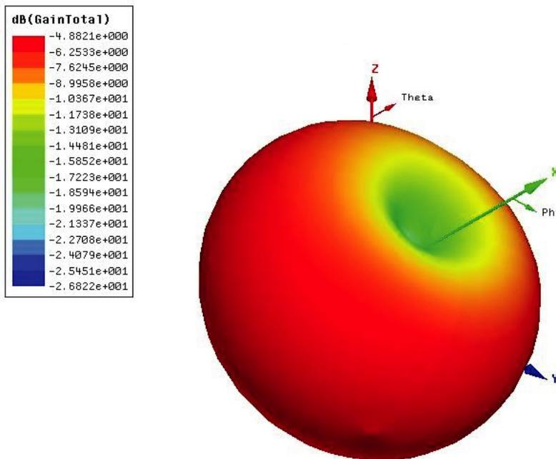
Fig. 3 - Simulated Radiation Pattern at 550 MHz
