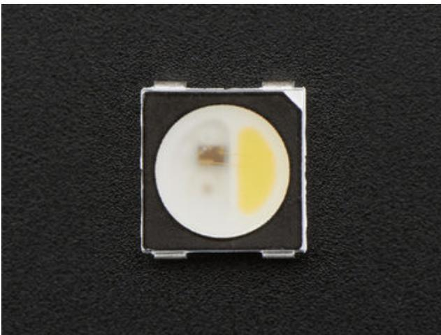
All measure 5 millimeters square. Adding a **0.1  $\mu$ F capacitor** between + and ground is recommended for each pixel.
