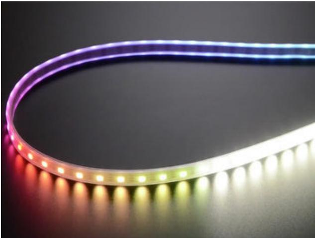
With a fourth LED per pixel, these strips may potentially draw up to 33% more current than their RGB equivalents. The maximum brightest cases are (approximately):
