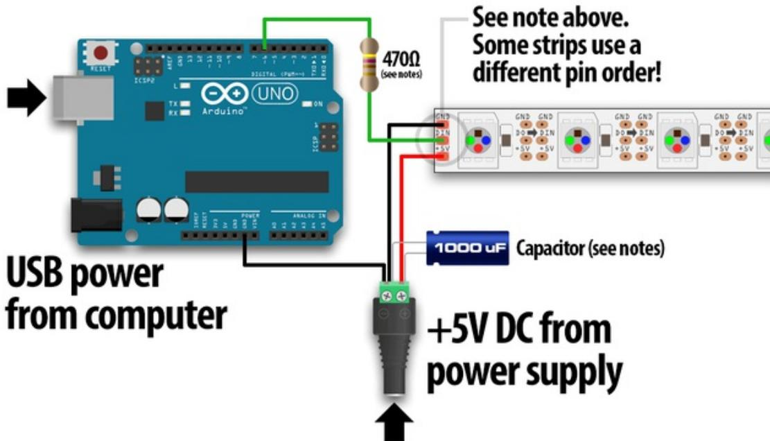
When connecting NeoPixels to any LIVE power source or microcontroller, ALWAYS CONNECT GROUND (–) BEFORE ANYTHING ELSE. Conversely, disconnect ground last when separating. When using a DC power supply, or an especially large battery, we recommend adding a large capacitor (1000 µF, 6.3V or higher) across the + and – terminals. This prevents the initial onrush of current from damaging the pixels. See the photo on the next page for an example.
