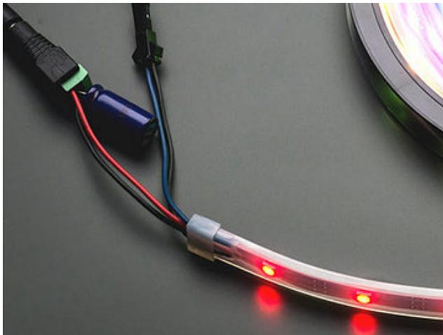
**Before connecting a NeoPixel strip to ANY source of power, we very strongly recommend adding a large capacitor (1000  $\mu$ F, 6.3V or higher) across the + and – terminals. This prevents the initial onrush of current from damaging the pixels.**
