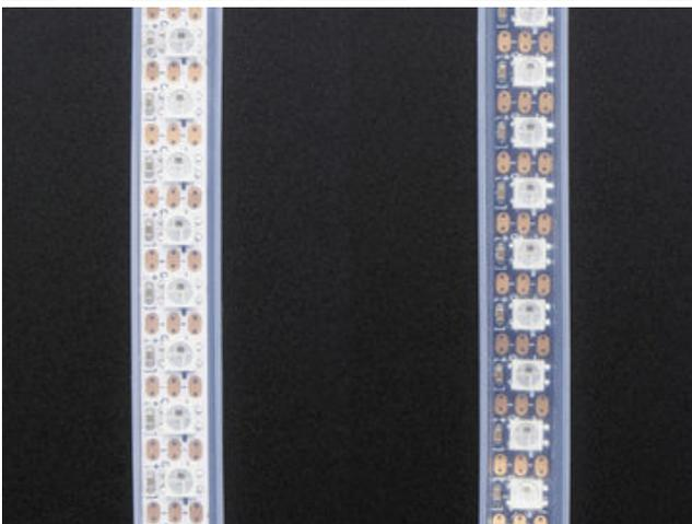
30 and 60 LED/meter strips are 7.5 mm wide, or 5 mm if you remove the strip from the casing (vs 12.5 mm / 10 mm for classic strips). The high-density 144/m strips are about 10 mm wide, or 7.5mm with the casing removed.
