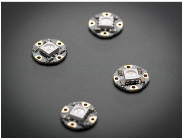
The original Adafruit NeoPixel form factor! **Flora RGB Smart NeoPixels** were designed for wearable projects using conductive thread, but can also be soldered normally with wires. These are available in two formats:
