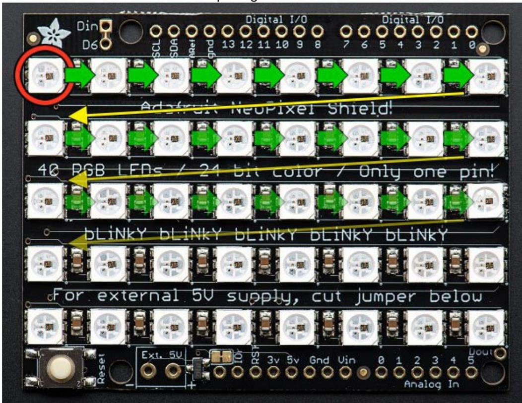
We refer to this layout as *row major* and *progressive*. *Row major* means the pixels are arranged in horizontal lines (the opposite, in vertical lines, is *column major*). *Progressive* means each row proceeds in the same direction. Some matrices will reverse direction on each row, as it can be easier to wire that way.
