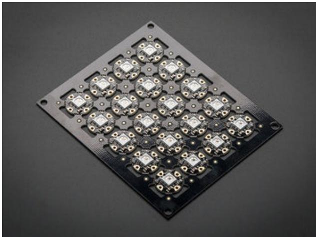
Flora RGB Smart Pixels measure about 12.5 millimeters (0.5 inches) in diameter. These are **RGB** only; there's no RGBW version.
