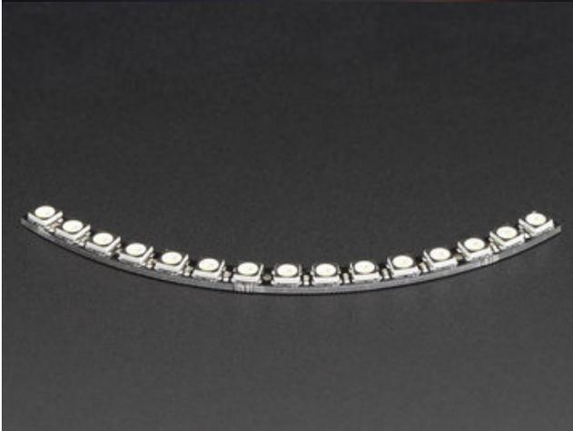
Though originally designed to be used in groups of four to complete a **60 NeoPixel Ring**, the individual **15-pixel quarter rings** can also be used to solve interesting design problems! **RGB** and **RGBW** are available.
