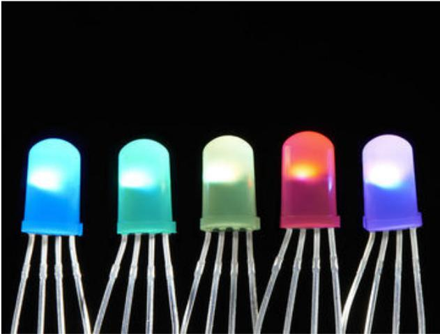
Through-hole NeoPixels are **RGB** only; there's no RGBW version. Use of a **0.1  $\mu$ F capacitor** (<http://adafru.it/753>) between + and ground on each pixel is strongly encouraged.
