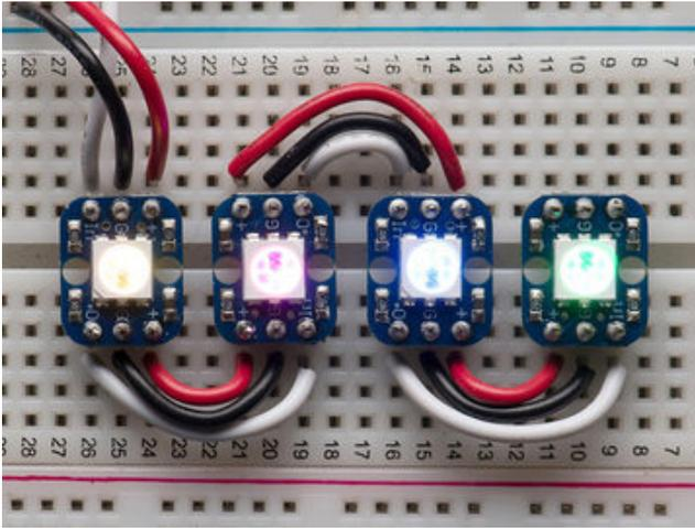
These are similar to the sewable Flora NeoPixels, but with a pin arrangement that (with the addition of headers) fits neatly into a breadboard for prototyping. Also available in two formats:
