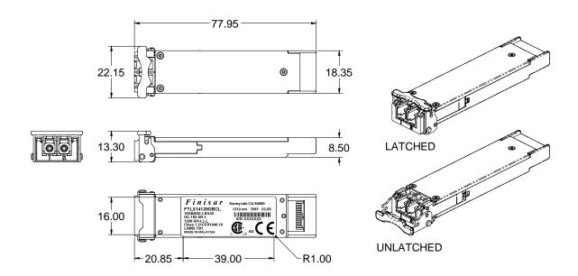
XFP Transceiver (dimensions are in mm)
