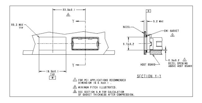
XFP Recommended Bezel Design (dimensions are in mm)
