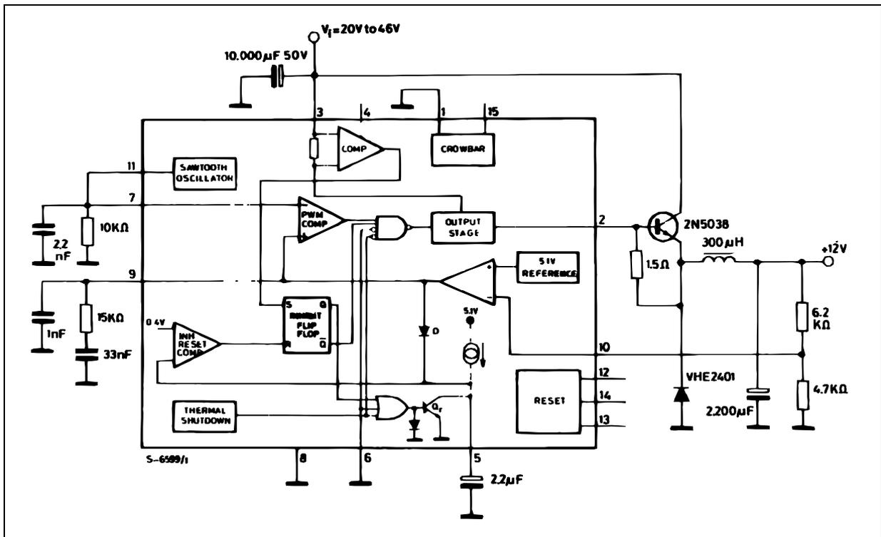
Figure 38 : Programmable Power Supply.
