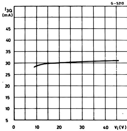
**Figure 8 :** Quiescent Drain Current vs. Supply Voltage (100 % Duty Cycle see fig. 6a).
