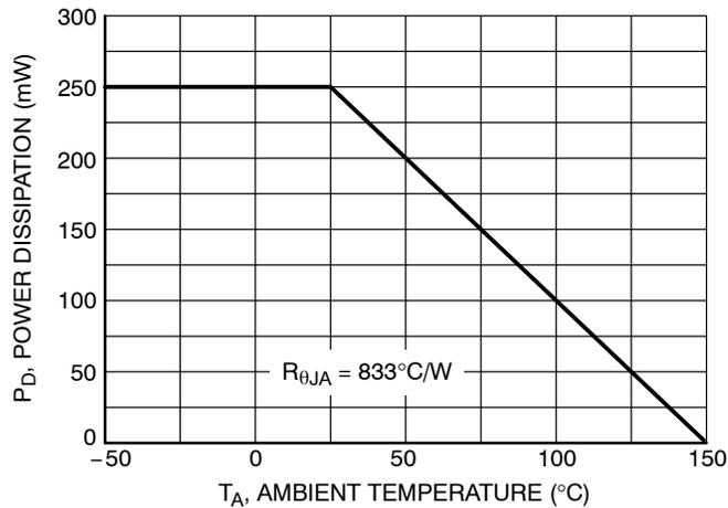
**Figure 1. Derating Curve**
