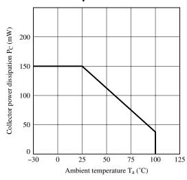
Fig.3 Diode Power Dissipation vs. Ambient Temperature
