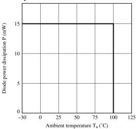
Fig.5 Total Power Dissipation vs. Ambient Temperature
