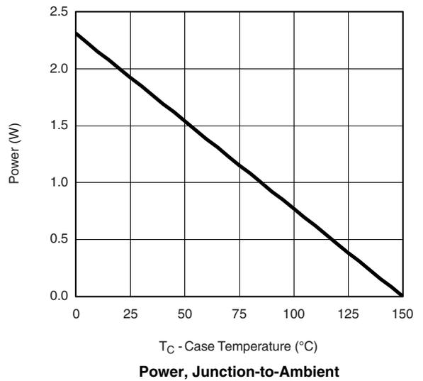
\* The power dissipation  $P_D$  is based on  $T_{J(max)} = 175$  °C, using junction-to-case thermal resistance, and is more useful in settling the upper dissipation limit for cases where additional heatsinking is used. It is used to determine the current rating, when this rating falls below the package limit.
