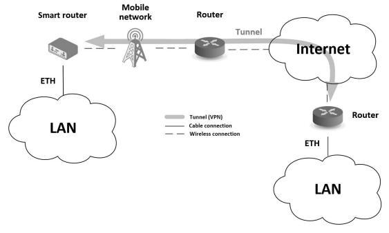
Figure 3: Using a VPN tunnel
