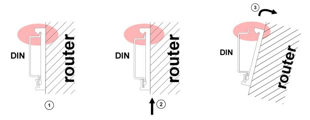
Figure 11: Removal of the DIN Rail
