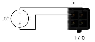
Figure 14: Connection of power supply
