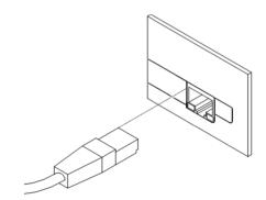
Figure 18: Connection of Ethernet cable
