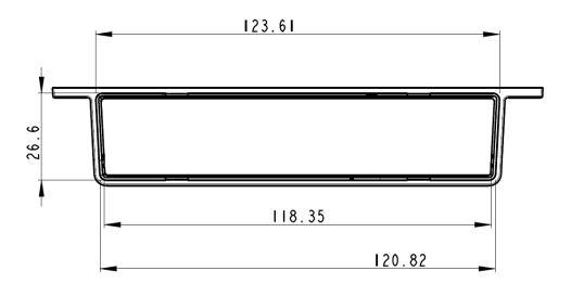
Figure 9: Basic dimensions of the router box
